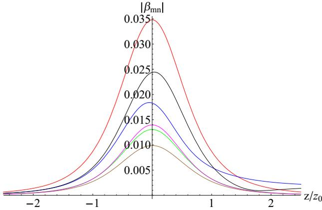
FIG. 2. (Color online) Absolute value of the coefficients of the higher transverse modes  $m + n \leq 6$  as a function of  $z$ , for  $y$ -polarized modes.  $\xi_L = \xi_T$  is assumed and the vertical axis is in units of  $\frac{A^3 k^3 c}{z_0^2}$ . Curves, from top to bottom:  $u_{11}$ ,  $u_{13}$ ,  $u_{31}$ ,  $u_{15}$ ,  $u_{33}$ ,  $u_{51}$ .
