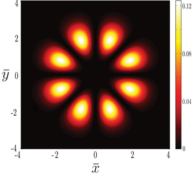
FIG. 4. (Color online) Normalized angular distribution of  $y$ -polarized photons at  $z \gg z_0$ , given by  $\frac{1}{2}|u_{13} - u_{31}|^2 \approx \frac{4}{3\pi} e^{-(\bar{x}^2 + \bar{y}^2)} \bar{x}^2 \bar{y}^2 (\bar{y}^2 - \bar{x}^2)^2$ .
